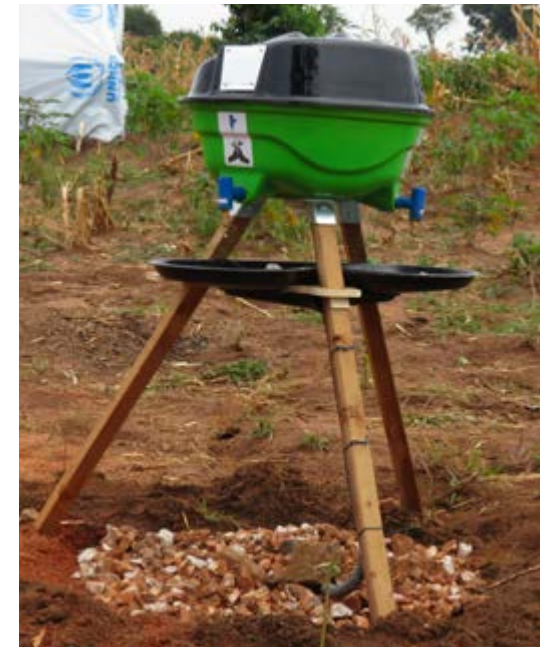
Image description: A handwashing station with two taps stands on three legs straddling a pit filled with gravel. Credit: Oxfam GB.
