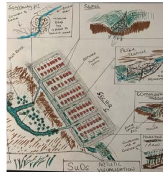
Image description: A sketch showing design features of the sustainable drainage project. Credit: Coventry University.
